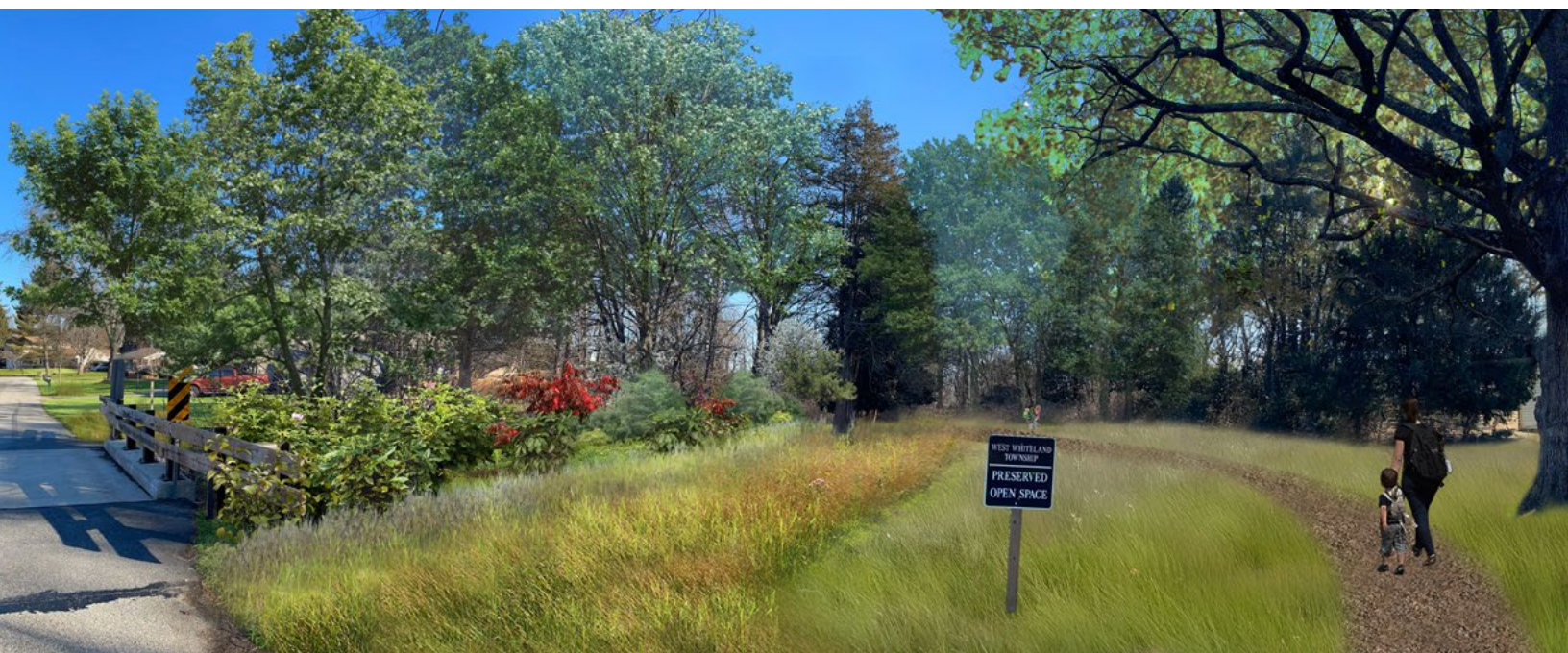
Located within the Valley Creek floodway, the homes on Locust Lane were purchased by the Township through the federal Hazard Mitigation Grant Program, with homeowner approval, demolished, and preserved as protected open space. This graphic illustrates the condition in 2025 and a photo-simulation of the properties with turf lawns converted to meadows and reestablishment of a riparian buffer.
